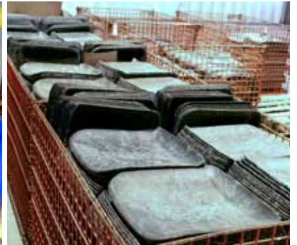
The IRT process begins with bales of unsorted plastic trash. Davidson chops the plastic into a fine, even consistency before the Kinetic Energy Melter converts the material into a molten resin. The resin is cured and formed into a final product.
