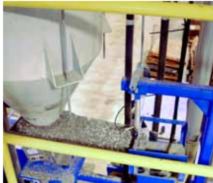
The IRT process begins with bales of unsorted plastic trash. Davidson chops the plastic into a fine, even consistency before the Kinetic Energy Melter converts the material into a molten resin. The resin is cured and formed into a final product.
